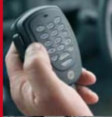
The TM8254's hand-held control head allows the angle and distance of the display to be positioned by the user for more accurate communication.
