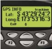
View on-screen GPS location information when you enable the software feature and connect the radio to a GPS receiver.
